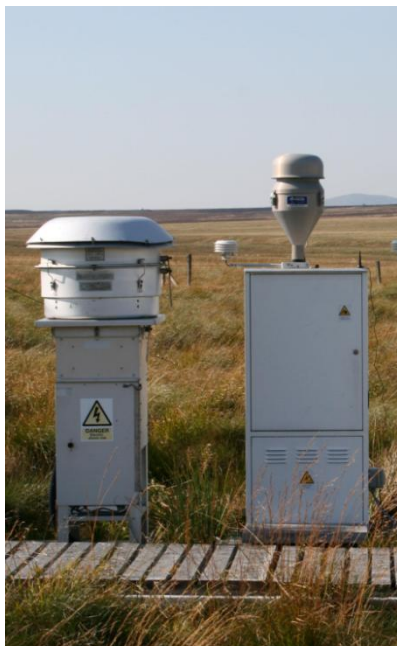
Figure 3. Andersen GPS-1 (left) and Digitel DHA-80 samplers at Auchencorth Moss, similar to the samplers used at Scunthorpe Town and Harwell.
